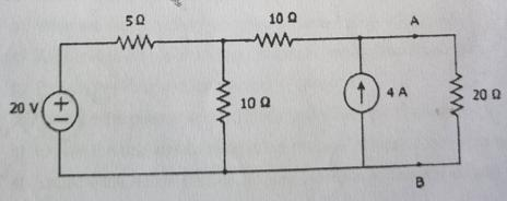
(a) State and explain superposition theorems .What are the limitations of Superposition theorem?
